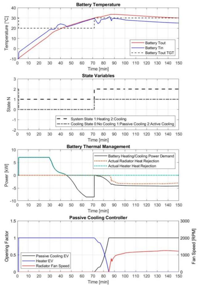
Figure 10 - Case A-10 Battery Heating and Passive Cooling
