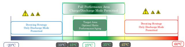
**Figure 1 - Battery Pack Operative Temperature**
