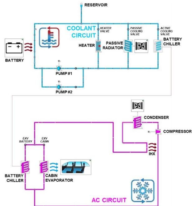
Figure 2 - Cooling System Layout
