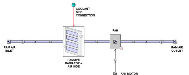
Figure 3 - Passive Cooling Branch / Air Side
